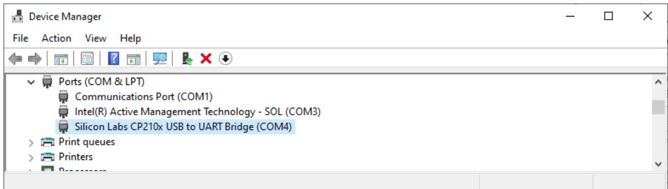
Fig. 1 USB-UART bridge installed
