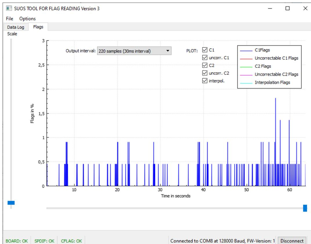
**Fig. 11 CFLG-Graph of a good disc**
